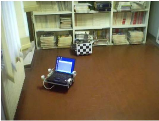
Fig. 7. Experimental set: MR follows the wall and brings the chess board pattern while OR localizes it and builds the map.
