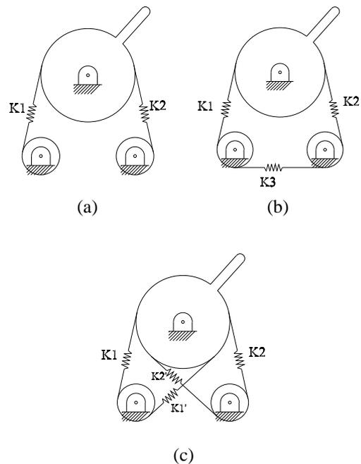
Fig. 1. (a) The simple antagonistic arrangement , (b) the arrangement with cross-coupling and (c) the bi-directional.
