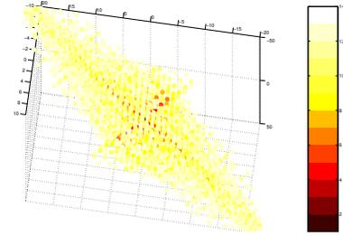
Fig. 5. Nodes with optimal cost less or equal than 11 represented on the fiber space for the 2-Trailer system (a scale of 2 on first component, of 6 on second component and of 24 on third component have been used)
