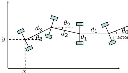
Fig. 3. A 3-Trailer system, in this case  $n = 6$ .
