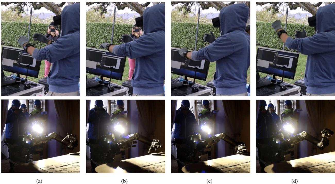
Fig. 11. A detail of a manipulation task executed during the field test. On the top line the pilot station is visible, with the operator wearing the Oculus and Myo bracelets, while in the bottom line the robot WALK-MAN executes the commanded actions.
