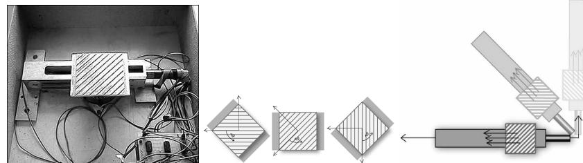
**Fig. 1.** Experimental apparatus for experiment 1: physical appearance (left); changing the pad texture orientation (middle); changing the slide orientation (right).
