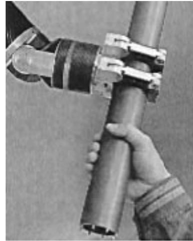
Fig. 2. Example of power grasping (courtesy of Barret Technologies, Inc.).
