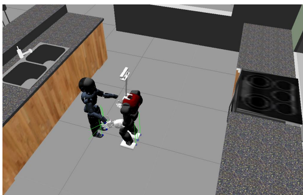
Figure 2: COMAN and iCub interacting inside a Gazebo simulation of a kitchen. Blue dots represent contact points.
