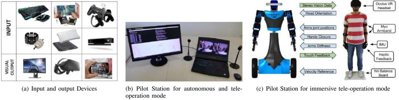
Fig. 4. (a), ALTER-EGO’s input and output interfaces. (b) and (c), autonomous and immersive tele-operation pilot station configurations.
