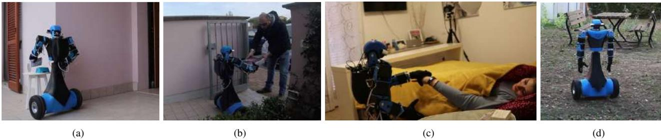
Fig. 8. (a) and (b), the robot is tele-operated to prepare food for pets and to retrieve a box from a mail man. (c), a pilot's relative is assisted by ALTER-EGO. (e), the robot is operated in an outdoor terrain characterized by the presence of small rocks, grass roots and a slight descent.
