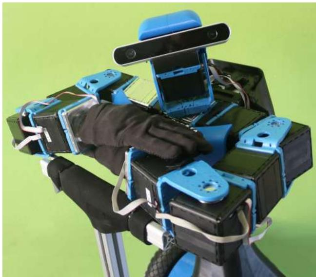
Fig. 1. ALTER-EGO, a soft dual-arm mobile platform equipped with variable stiffness actuation units and soft under-actuated hands.
