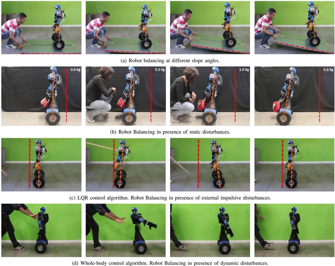
Fig. 6. (a) and (b) show the balancing behavior of the robot in presence of changes in the slope angle of the floor and static disturbances. (c) and (d) show the balancing performance (in presence of dynamic disturbances) with the LQR and the whole body controllers developed.
