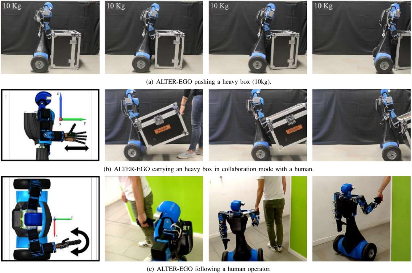
Fig. 5. Autonomous actions: pushing an heavy object (a), carrying a box in collaborative mode (b), and following a human operator (c).
