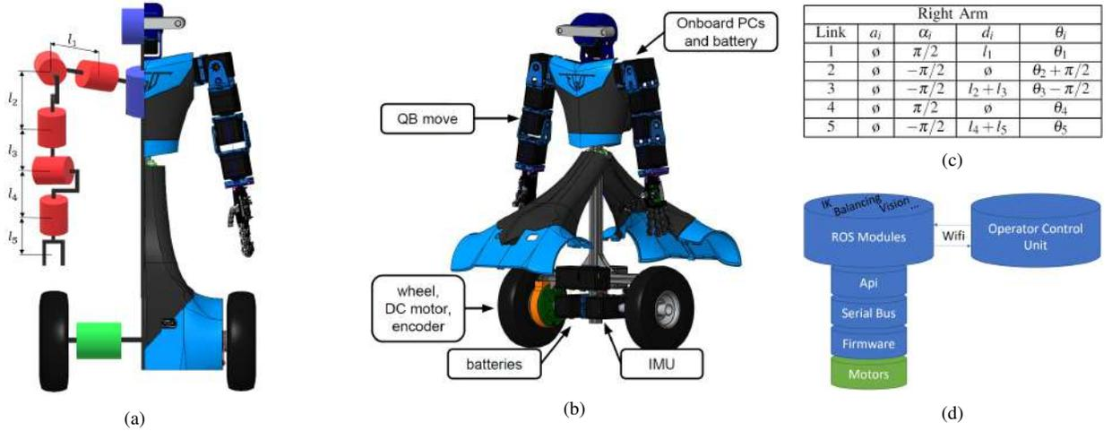
Fig. 2. (a) and (b) show the mechatronic architecture of ALTER-EGO. (c) and (d) show Denavit-Hartenberg parameters of arms, and the overall software architecture.  $l_i$  represents the length of  $i$ -th link,  $a_i, \alpha_i, d_i, \theta_i$  are the Denavit-Hartenberg parameters of the  $i$ -th link [10]
