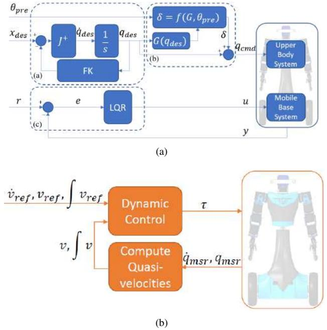
Fig. 3. ALTER-EGO Control Schema. The full state feedback control system obtained with LQR is reported in (a). The Whole-Body control schema is showed in (b).
