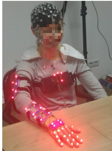
Fig. 2: Exemplary experimental set-up. The subject is equipped with high resolution EEG sensors and active optical markers for motion tracking.
