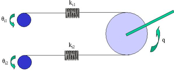
Figure 1: An antagonistic arrangement of two actuators per joint with nonlinear springs can control joint position and stiffness independently.
