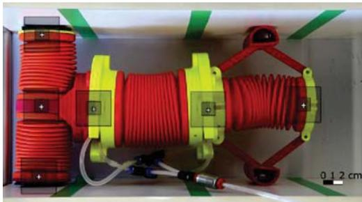
Fig. 12. Markers positions for the analysis in the Kinovea software suite.
