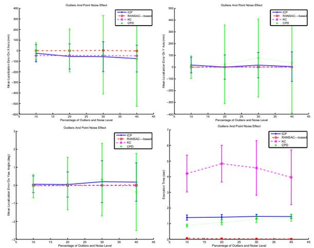
Fig. 1. Accuracy on the  $X_w$  and  $Y_w$  axis (in millimeters, upper row), accuracy of the orientation angle (in degrees, bottom row, left) and the execution time (in seconds, bottom row, right). The effect of both noise (drawn from a Gaussian distribution with increasing standard deviation from 0mm to 40mm) and outliers (with a percentage from 0% to 40%) are reported.
