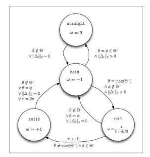
Fig. 8. Finite state automaton that summarizes the collision avoidance protocol GRP.
