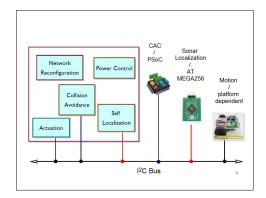
Fig. 12. Hardware Expansion Layout. All external hardware communication is performed by I2C bus sharing.
