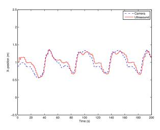
Fig. 4. X-position estimate generated by the ultrasound system (solid) together with measurements from a camera system (dashed). Data is logged every 1200 ms.
