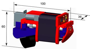
Fig. 2: W-FYD CAD design. Dimensions are in mm and the total mass is 100 g.
