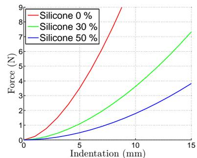
Fig. 7: The  $F(\delta)$  characteristics of the three silicone specimens used for the experiments with humans. Silicone 0% corresponds to SS1, while Silicone 30% and Silicone 50% can be referred to as SS2 and SS3, respectively.
