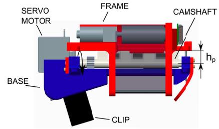
(a) Lifting mechanism and finger interaction in passive mode.
