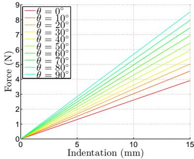
Fig. 6: Elastic fabric force indentation characterization.
