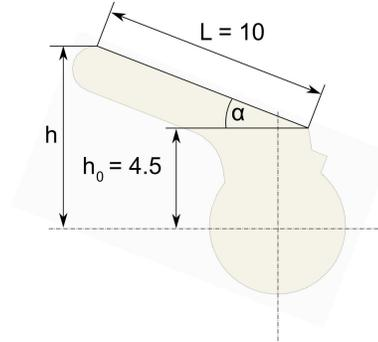
(b) Lifting mechanism: cam profile. Dimensions in mm.
