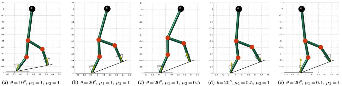
Fig. 3. In panel (a) is represented the optimized configuration of a humanoid robot approaching a surface with inclination  $\theta = 10^\circ$ , with friction coefficients  $\mu_1 = \mu_2 = 1$ . Panels (b)–(e) show the result of the optimization for a surface with inclination  $\theta = 20^\circ$ , varying the friction coefficients.
