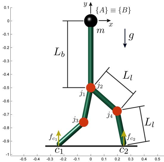
Fig. 2. A humanoid robot upright in a vertical plane. The robot is touching the floor with the feet, on a plane with variable inclination and friction.
