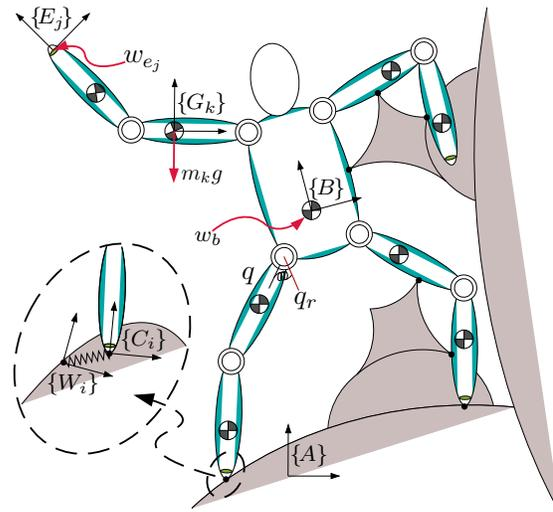
Fig. 1. Reference scenario for the description and the analysis of *whole-body loco-manipulation* tasks with humanoid robots.
