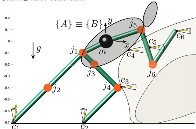
Fig. 4. A humanoid robot pushing a heavy object in a typical *whole-body loco-manipulation* task.
