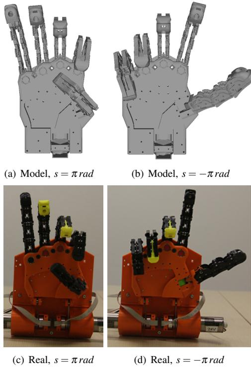
Fig. 10. Postures of the Pisa/IIT SoftHand+, model versus experimental. The posture correspond to a constant value of  $\sigma = \pi \text{ rad}$  and two different values of  $s = \pm\pi \text{ rad}$ . Postures forecast by the model in simulation (top row) are compared with experimental results (bottom row).
