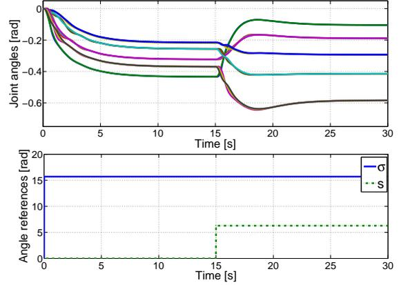
Fig. 5. Simulated joint angles evolutions on the SoftHand+. The system inputs are a step of  $5\pi rad$  along the first DOA  $\sigma$  at time 0s, then another step on the second DOA  $s$ , with amplitude  $2\pi rad$  at time 15s (abduction angles omitted for clarity, negative angles corresponds to hand closure).
