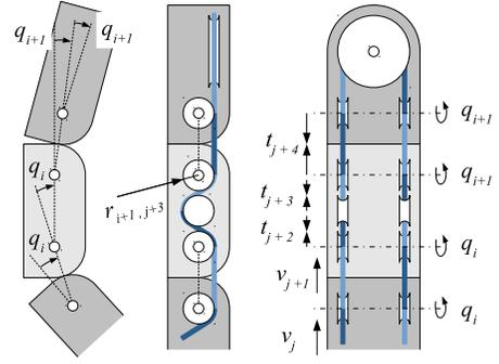
Fig. 4. Scheme of a finger of the SoftHand+ with main variables indicated.  $q_i$  is the  $i$ -th joint angle,  $v_j$  and  $T_j$  are the speed and tension, respectively, of each segment of tendon along its routing,  $r_{j,i}$  is the radius of the  $j$ -th pulley when it is on joint  $i$ , or 0 otherwise.
