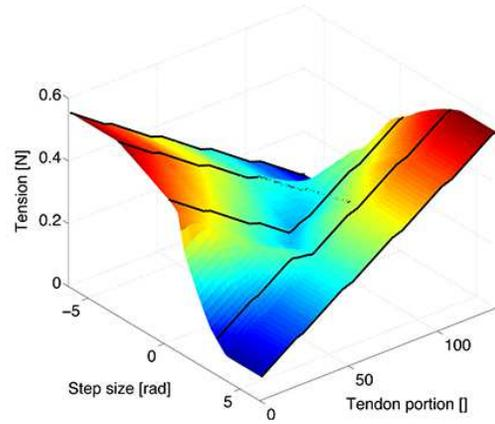
Fig. 8. Steady-state tensions distributions on the tendon with respect to changing amplitude of step input  $s$ . Results are obtained in 26 independent simulations. Each simulation step size differs of  $\frac{\pi}{6} \text{rad}$  from neighboring simulations. Tension distributions generated by step of  $-2\pi$ ,  $-\pi$ ,  $0$ ,  $\pi$ , and  $2\pi \text{rad}$  are highlighted with black lines.
