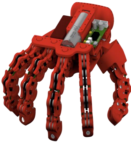
Figure 1 A preliminary prototype of synergy-inspired hand developed
