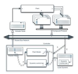
Figure 1: The proposed control architecture
