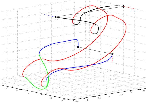
Fig. 7. Path obtained from  $\mathbf{q}_s = (0, 0, 0, 3, 0, 0)^T$  (stars) to  $\mathbf{q}_f = (0, 0, 4, 0, 3, 4)^T$  (diamonds) with  $\mathbf{v}_1(t_0) = (0, 0, 1)^T$ ,  $\mathbf{v}_2(t_0) = (0, 0, -1)^T$ ,  $\mathbf{v}_1(t_f) = (-1, 0, 0)^T$  and  $\mathbf{v}_2(t_f) = (1, 0, 0)^T$ . Furthermore, a maximum control magnitude of 1 as been considered.
