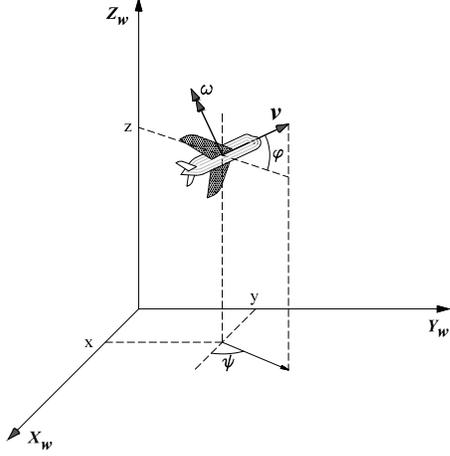
Fig. 1. Representation of a vehicle in a 3D space
