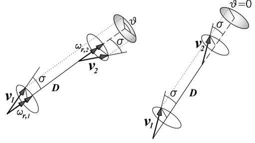
Fig. 3. Steering  $\theta$  to zero (keeping constant  $\sigma$ )
