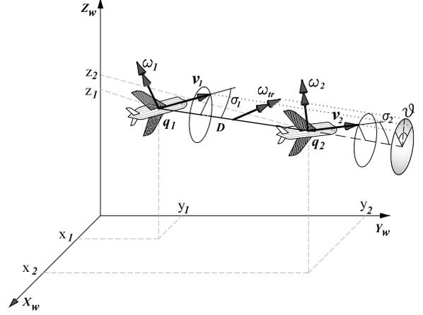
Fig. 2. Configuration of the *3D-Dubins* system
