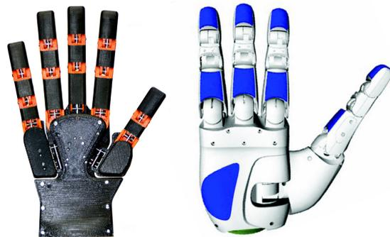
Fig. 1. Different multi-fingered robotic hand designs. The left image corresponds to THE first hand developed at the Centro E. Piaggio with five fingers, and the right image corresponds to the Schunk Anthropomorphic hand, based on the DLR II hand, with four fingers
