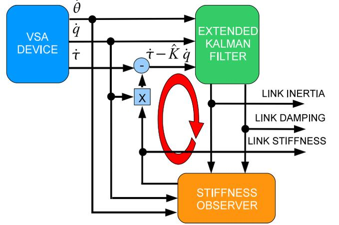
Fig. 2. Schematic of the observer as proposed in section III-A. The interaction loop between the two observers is highlighted.
