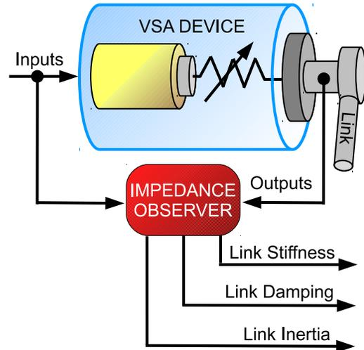
Fig. 1. Concept of impedance observer for a variable stiffness robot: inertia, damping and stiffness on the link side are estimated from measures of inputs (motors currents) and outputs (angles and torques) of VSA device.
