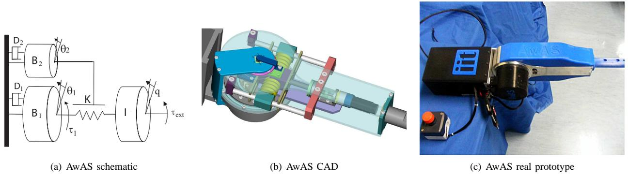
Fig. 3. The Actuator with Adjustable Stiffness (AwAS) used as a testbed for the proposed impedance observer. Schematic (a), CAD image (b) and prototype (c).
