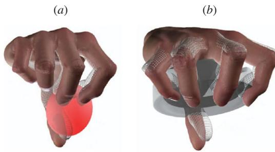
Figure 4. Application of the soft synergy model to the grasp of a cherry-like object (*a*) and of an ashtray (*b*). In wireframe is the reference hand, moving according to the constraint manifold corresponding to the first three synergies.
