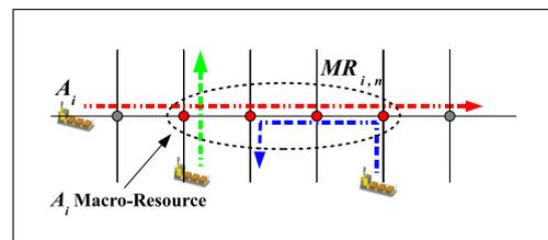
Fig. 3. Example of a macro resource shared partially with multiple AGV
