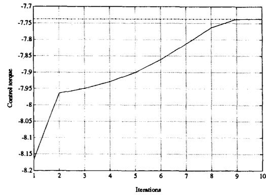
Figure 5: Plot of control torque history starting from an over-estimate of optimal contact forces.
