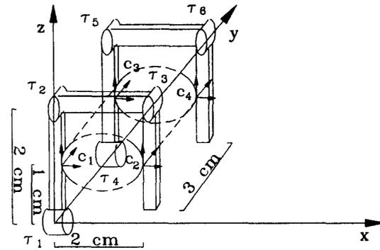
Figure 6: Power grasp with a two fingered hand.
