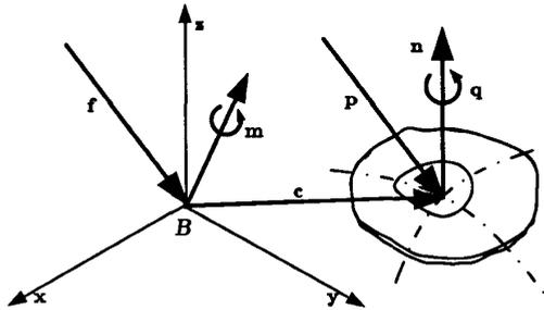
Figure 3: Knowns (force and torque measurement vectors  $\mathbf{f}$  and  $\mathbf{m}$ ) and unknowns (contact centroid location  $\mathbf{c}$ , contact force  $\mathbf{p}$  and spin torque  $\mathbf{q}$ ) of the problem.
