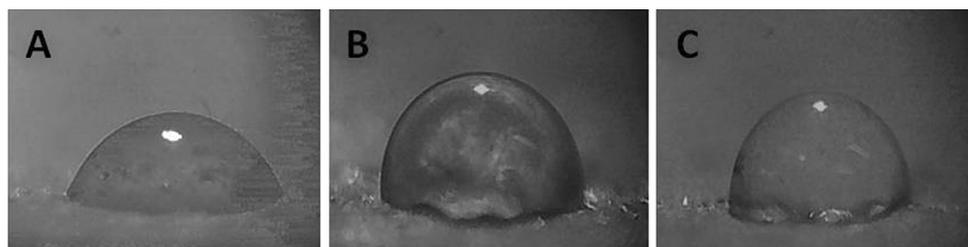
**Fig. 6** Water droplet images captured immediately after droplet deposition on blue paint replicas (a), on paint replica coated with fresh Disboxan 450<sup>®</sup> (b), and on blue paint replicas coated with Disboxan 450<sup>®</sup> after two years of natural outdoor ageing (c)
