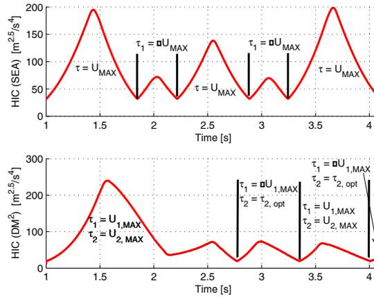
**Fig. 6.** Maximum of the HIC value in various failure cases for SEA (top) and DM<sup>2</sup> (bottom).
