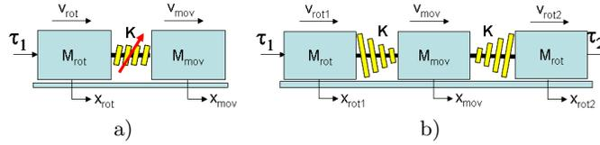
**Fig. 1.** The concept of Variable Impedance Actuation (a) and a possible implementation by means of antagonistic actuators (b). Effective rotor inertias are coupled to the link inertia through nonlinear springs.
