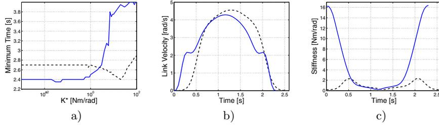
**Fig. 4.** a) Minimum time to reach the target configuration vs. cross-coupling stiffness  $K_3$  ( $L_0 = 1$ ). Solid:  $\sigma_0 = \sigma_f = 16$  Nm/rad; dashed:  $\sigma_0 = \sigma_f = 0.2$  Nm/rad. Optimization results for antagonistic actuation with cross-coupling in a pick-and-place, stiff-to-stiff task (solid) and soft-to-soft task (dashed): velocity (b) and joint stiffness (c).
