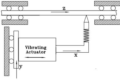
Fig. 14. A micro-electro-mechanical (M.E.M.) motion rectifier illustrating the definition of external nonholonomy in a piecewise holonomic system.
