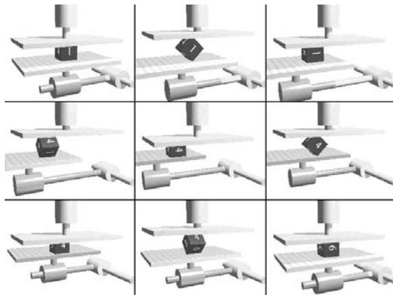
Fig. 1. A die being rolled between two movable parallel plates. The plates can be thought of as the jaws of a robotic gripper, manipulating the polyhedron for reorientation purposes. The sequence illustrates a behaviour which could be qualitatively described as nonholonomic.
