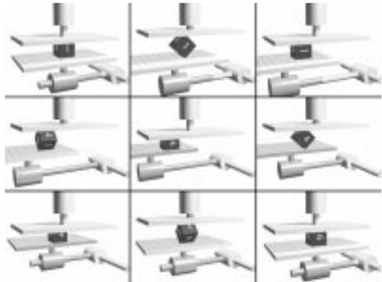
Fig. 1. A parallel-jaw gripper with three d.o.f. can manipulate polyhedral parts. Plates are covered by compliant, high-friction pads. Vertical motion is passively controlled so as to accommodate for the changing height of parts while keeping suitable grasping forces.
