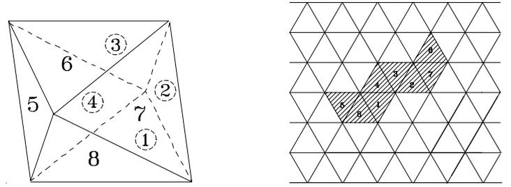
Fig. 3. An octahedron and its development on the plane. Circled numbers refer to hidden faces.
