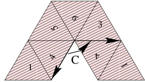
Fig. 4. For the development on the plane of a octahedron, the sequence (1, 4, 5, 6, 3, 4, 1) produces a rigid rotation of an angle  $2\pi/3$  about point  $C$ .
