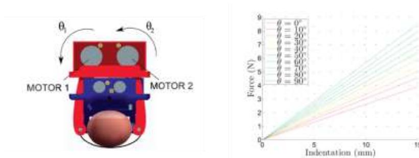
**Fig. 4.** Representation of a finger interacting with the W-FYD (on the left); characterization curves for different motor positions ( $\theta_1$  and  $\theta_2$ ) (on the right).
