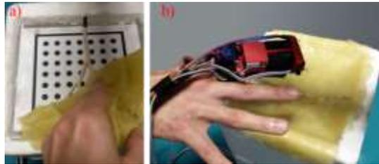
**Fig. 9.** Experimental set-up: a) sensorized arterial tree covered with synthetic connective tissue and positioned over a box (with the calibration grid). b) a surgeon wearing the W-FYD.
