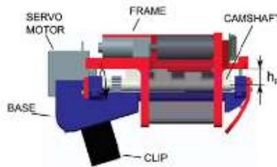
**Fig. 5.** Passive Mode: the fabric frame is put in contact by the camshaft lifting mechanism and servo-motor, inducing a variation of the height  $h_p$  of the frame.
