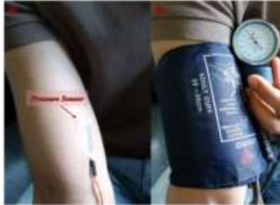
**Fig. 8.** Calibration procedure: a) positioning of the pressure sensor, b) manual sphygmomanometer used for the sensor calibration.
