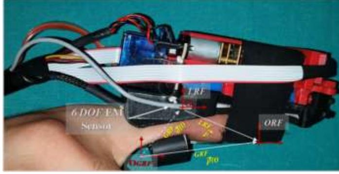
**Fig. 6.** W-FYD sensorized with a 6DOF EM Aurora Sensor
