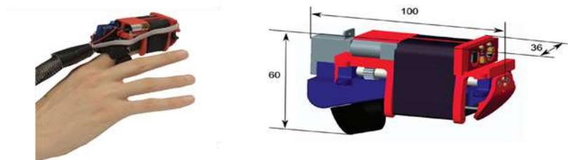
**Fig. 3.** W-FYD on a user's finger (on the left): W-FYD CAD design and dimensions (in mm) – weight 100 g.
