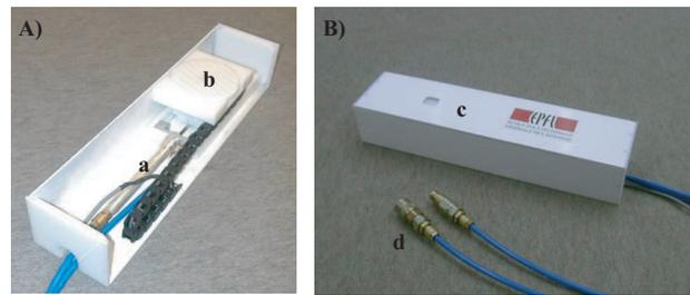
Fig. 2. The slave module. A) Without cover, showing the slave hydraulic piston (a) and the tactile pad (b). The ultrasonic motor is located beneath the tactile pad. B) The closed module showing the touch-pad (c) and the disconnectable (d) hydrostatic transmission.
