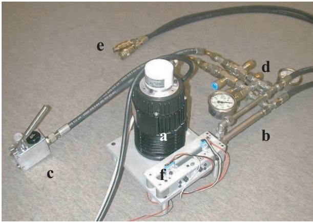
Fig. 4. The master actuator: DC torque motor (a), master hydraulic cylinder (b), hydraulic pump (c) and circuitry (d) as well as disconnectable hydrostatic transmission (e) and security switches (f).
