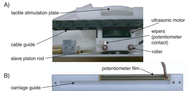
Fig. 3. A) Close-up view of the carriage in the slave module. The carriage is actuated by the slave piston and held by two lateral guides. The right guide (B) also holds the potentiometer film.
