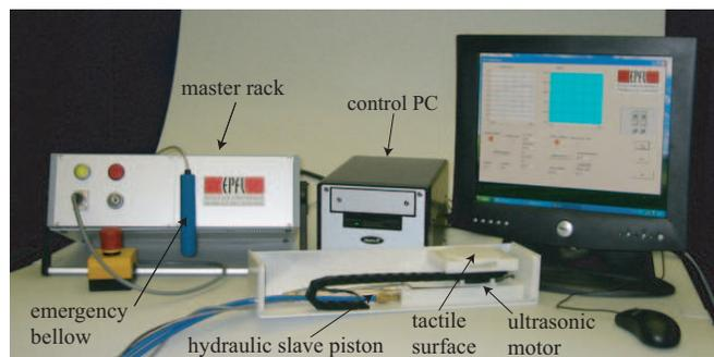
Fig. 1. MR compatible interface to investigate the brain mechanisms of tactile perception. The slave module, shown in the front, contains an active rotary degree of freedom (ultrasonic motor) linked to a translatory degree of freedom (brass hydraulic piston).
