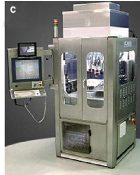
**Fig. 3.** Bioprinters: a) 3D dispensing Laboratory Bioprinter – ‘LBP’ (designed by Neatco, Toronto, Canada in cooperation with MUSC Bioprinting Research Center, Charleston, SC); b) 3D robotic printer – ‘Fabber’ (designed by Cornell University, USA); c) 3D robotic industrial bioprinter — ‘BioAssembly Tool’ (designed by Sciperio/nScript, Orlando, USA).
