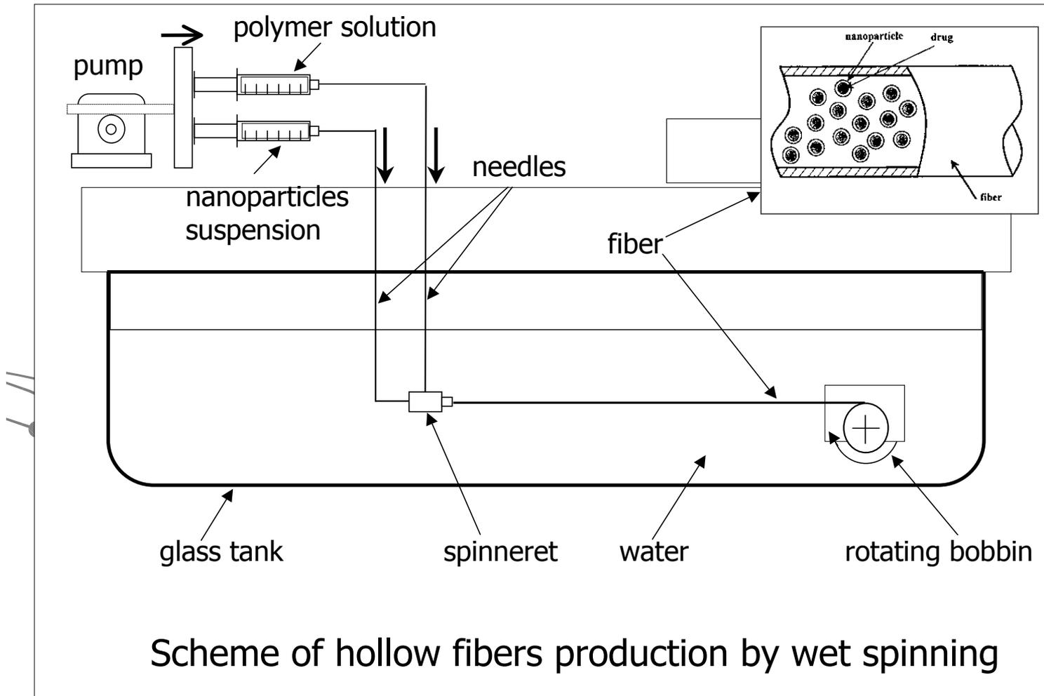
Scheme of hollow fibers production by wet spinning
