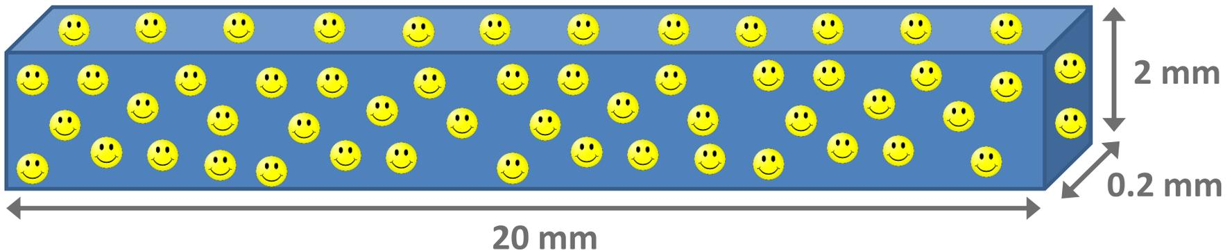
**Not implementable in real fluidic systems as it requires very high medium flow rates that damage cells due to high shear stresses**
