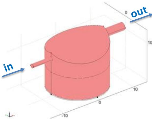
$$v_{in} = 3.82 \times 10^{-3} \text{ m/s} = 180 \text{ } \mu\text{L/min}$$
