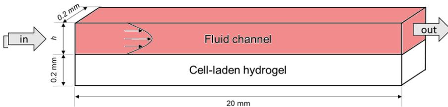
$$v_{in} = \frac{\tau_w \cdot h}{6\eta}, \quad \tau_w = 15 \mu\text{Pa}$$
