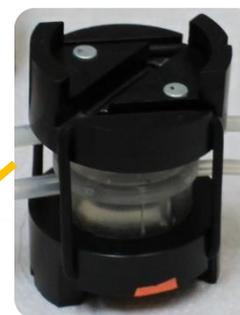
2 flow membrane bioreactor with realtime TEER
