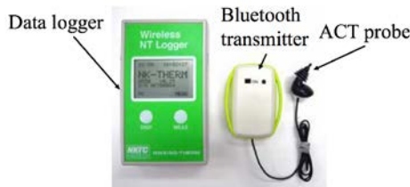
Fig. 2 The aural canal thermistor used in the study of temperature monitoring of a patient with spinal cord injury. The aural canal thermistor that we used is manufactured by Nikkiso-Therm Co.
