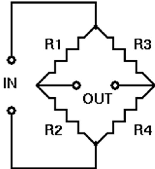
when  $R1/R2 = R3/R4$  →  $V_{out}=0$
