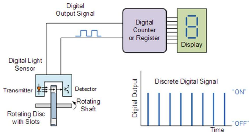
For example, the speed of the rotating shaft can be measured by using a digital LED/Opto-detector sensor.
