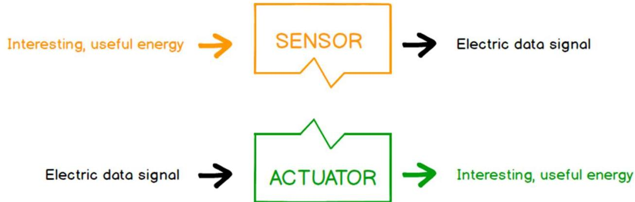
The word “**Transducer**” is the collective term used for both Sensors and Actuators.
