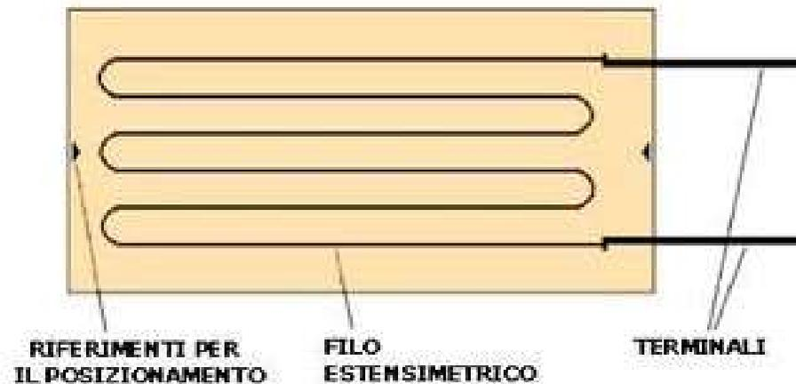
The sensitivity to strain is expressed quantitatively as the **gauge factor (GF)**, defined as the *ratio of fractional change in electrical resistance to the fractional change in strain*.
