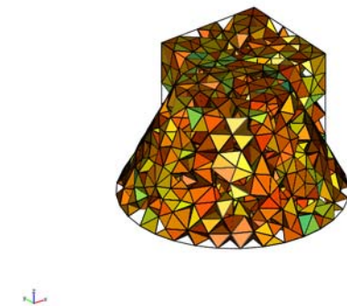
Element quality plot for a fraction of the elements
