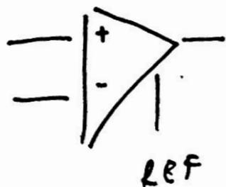
$$V_{out} = A \cdot (V^+ - V^-) + R_{EF}$$
