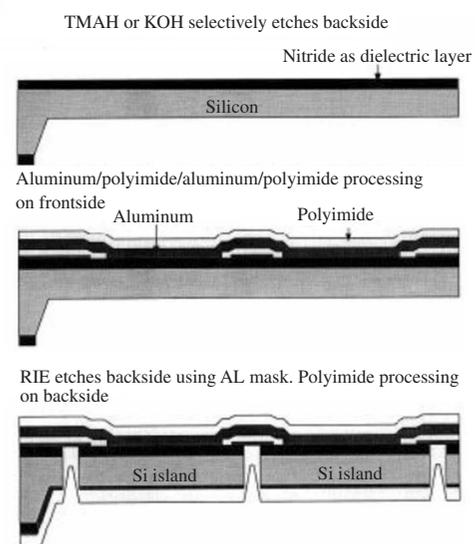
**Figure 4.** Wafer-size flexible skin based on MEMS technology. (Reprinted with permission from [122], F. Jiang et al., *Sensor. Actuat. A—Phys.* 79, 194 (2000). © 2000, Elsevier.)
