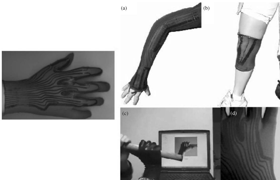
**Figure 5.** Truly wearable systems based on sensorized fabric. (Reprinted with permission from [82], F. Lorussi et al., *IEEE Sens. J.* 4, 807 (2004). © 2004, IEEE.)
