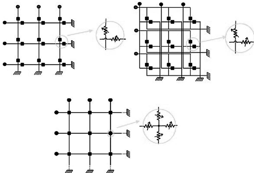
**Figure 6.** Several topologies used in sensor arrays: connection in series, parallel and net of quadruples. (Reprinted with permission from [83], D. De Rossi et al., "Proc. of IEEE Sensors," p. 1608. Orlando, FL, 2002. © 2002, IEEE.)
