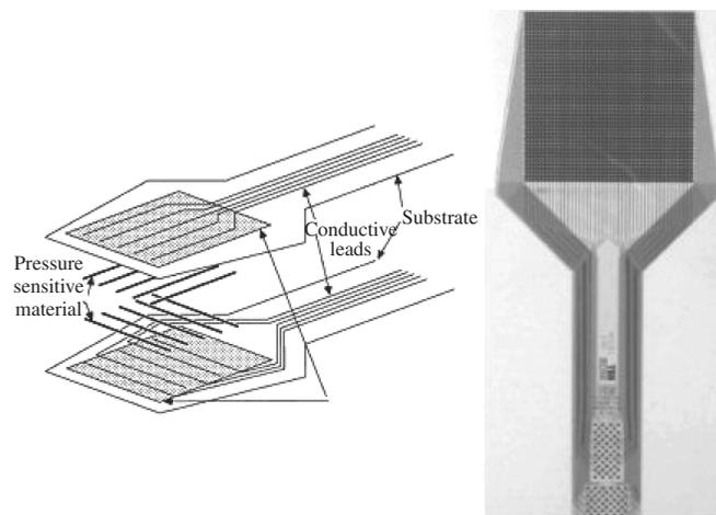
**Figure 3.** Flexible, thin-film contact resistive force and pressure sensors printed on polyester substrates manufactured by Tekscan Inc. (Reprinted with permission from [85], T. V. Papakostas et al., in “Proceedings of the 1st IEEE Sensors Conference,” Vol. 2, p. 1620. Orlando, FL, 2002. © 2002, IEEE.)
