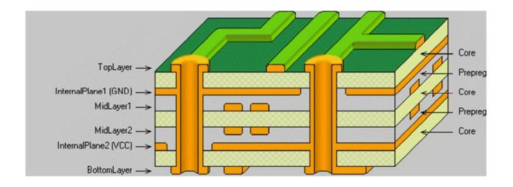
Your circuit design software will allow you to output the PCB layout in a format called **Gerber** with one file for each PCB layer (copper layers, solder mask, legend or silk) to allow manufacturing.
