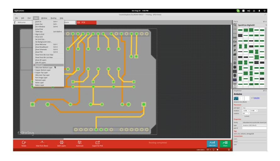
Especially for the PCB, it would be useful to **check it both from above and from below** before finalizing the positions of each part.
