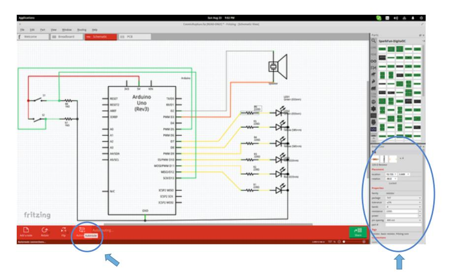
The parts feature **ports** are best shown in the "Schematic" view mode so that the user can comfortably connect what is needed.
