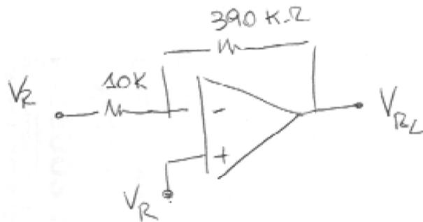
$$V_{RL} = V_R \left( 1 + \frac{390K\Omega}{10K\Omega} \right) - V_R \left( \frac{390K\Omega}{10K\Omega} \right)$$
