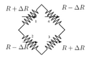
$$V_{out} = V_{ref} \frac{\Delta R}{R}$$
