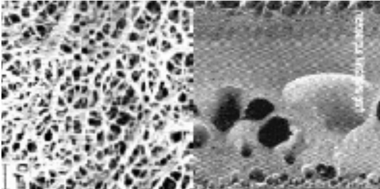
Wall with variable porosity obtained by filament winding
