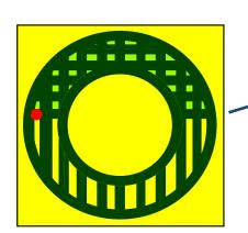
When cross section is complete, elevator indexes to prepare for next layer.
