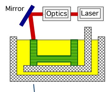
Laser is focused/shaped through optics. A computer controlled mirror directs laser to appropriate spot on photopolymer surface. Polymer solidifies wherever laser hits it.
