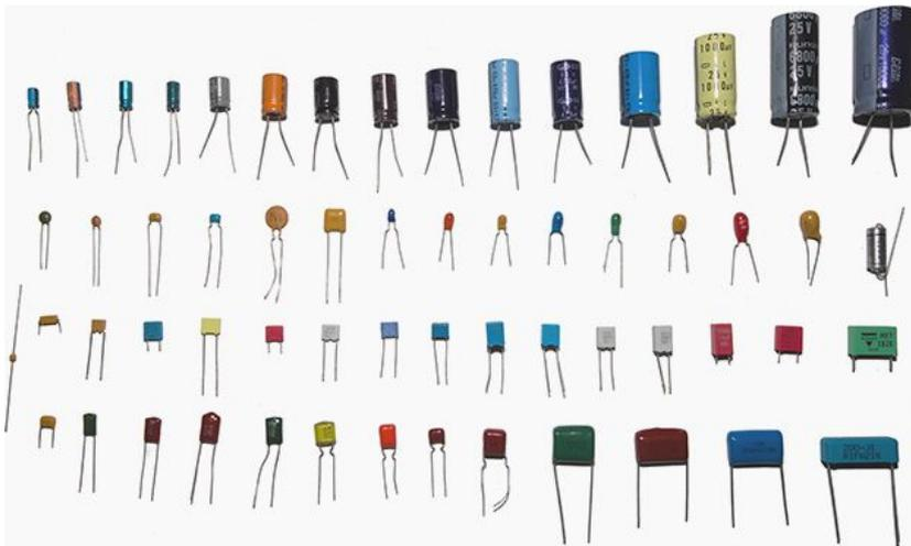
Basically a capacitor is formed *from two conducting plates separated by a thin insulating layer*. They are manufactured in many forms, styles, and from many materials. Capacitors are widely used in electrical and electronic circuits.
