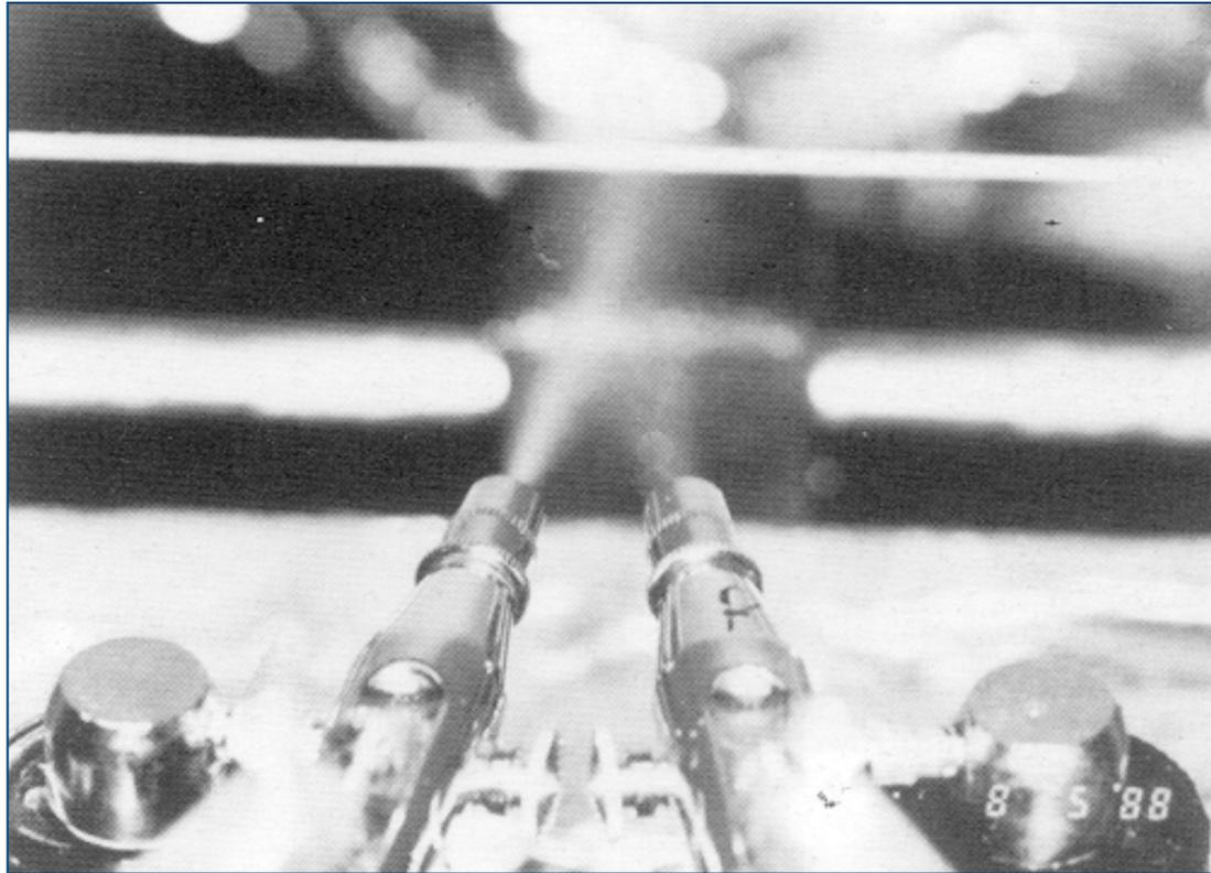
Two modified spray guns were mounted on the carriage and positioned vertically so that their nozzles were aligned with the longitudinal axis of the mandrel, at the distance and an angle from the mandrel such that the intersection of the jets occurred at the surface of the mandrel.
