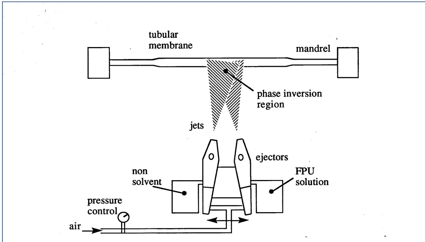
Scheme of the apparatus for the fabrication of tubular membranes
