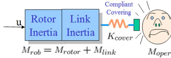
**Fig. 1.** Simplified model of the impact between a rigid 1DOF robot arm and an operator.
