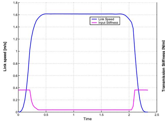
**Fig. 6.** Optimal joint stiffness and velocity during a rest-to-rest task under safety constraints, as obtained by a numerical solution to the safe brachistochrone of a VS actuator.
