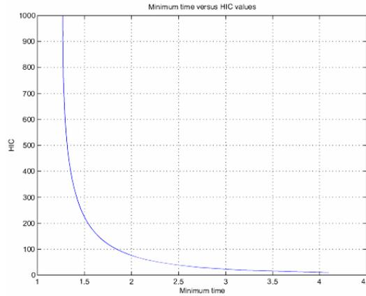
**Fig. 2.** The safety-performance tradeoff curve for the rigid single joint case.
