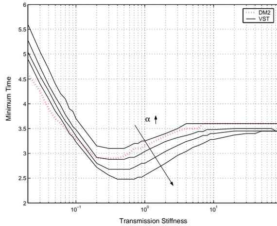
**Fig. 7.** Results of the safe brachistochrone for both VS transmission (*black*) and  $DM^2$  (*red*) schemes, as a function of the stiffness center value  $\bar{\sigma}$  and for different stiffness ranges  $\Delta\sigma$ . It is noteworthy that as large is the range of stiffness allowed for VS transmission, as large is the performance recovering (row means that  $\Delta\sigma$  increases for constant  $\bar{\sigma}$ ).
