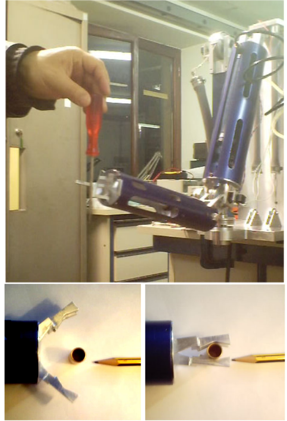
Figure 7: Robot picking a screwdriver (up) with the prototype of light gripper developed in our laboratory (bottom).
