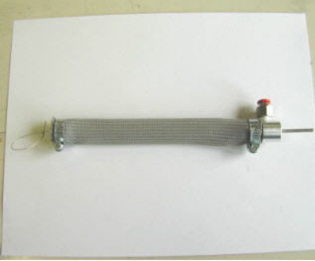
Figure 5: A McKibben pneumatic artificial muscle built in our laboratory.
