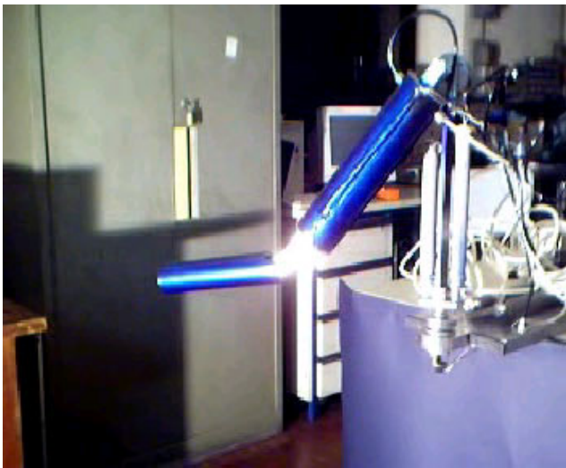
Figure 8: The Soft Arm is a lightweight structure actuated by McKibben artificial muscles in antagonistic pairs with an antropomorphic kinematics.
