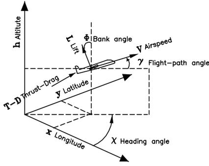
Figure 1: Aircraft coordinate system
