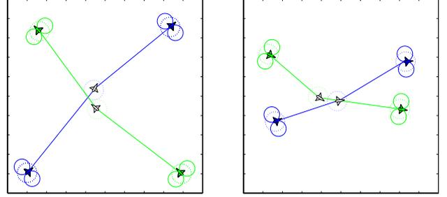
Figure 3: Numerically computed solutions to optimal cooperative conflict resolution for two aircraft. Minimum curvature circles are reported at the start and goal configurations, along with safety discs of radius  $d/2$  (dashed). Optimal solutions consist of two unconstrained Dubins' trajectories for each aircraft, pieced together with a zero-length constrained arc.
