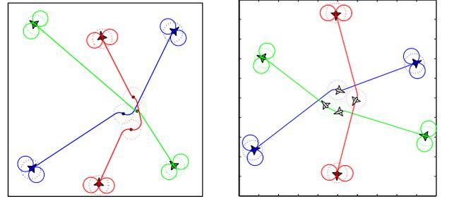
Figure 4: Two cases of three-aircraft conflict resolution. Left: a level 2 solution whereby the aircraft starting in the middle contacts first the one arriving on its right, and after the one arriving from left. Right: a level 2 resolution that generates a roundabout-like maneuver.
